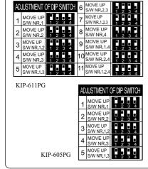
\*\* When using DS-4M(OPTION) with KIP-611PG or KIP-605PG it should be No.1 in DIP switch.
